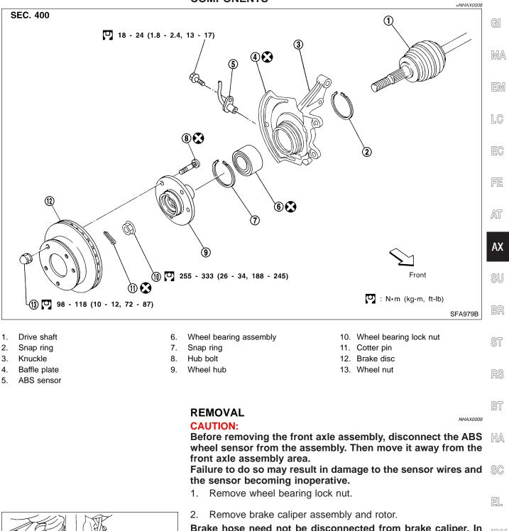
Brake hose need not be disconnected from brake caliper. In this case, suspend caliper assembly with wire so as not to stretch brake hose. Be careful not to depress brake pedal, or piston will pop out.
